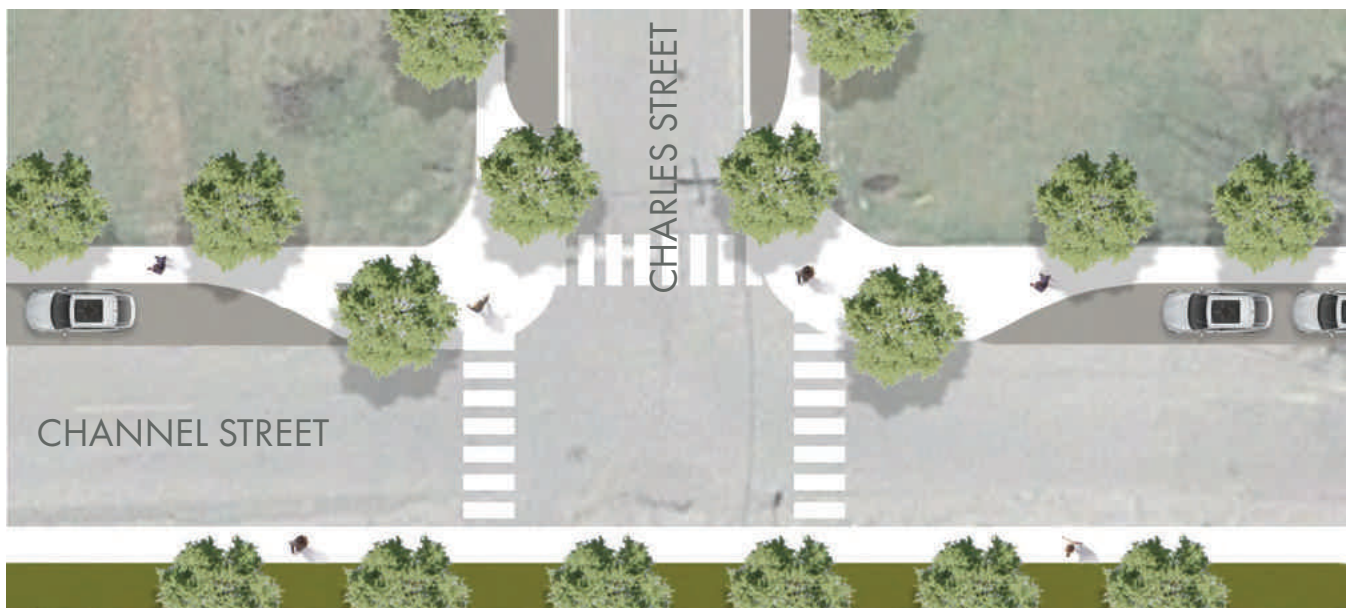
Example of creating a more defined crossing at the intersection of Charles Street and Channel Street.
