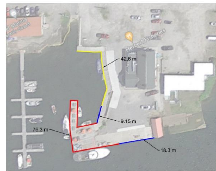
EXISTING MOORING LENGTH SCALE: 1:750
